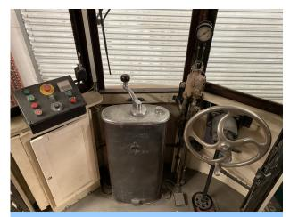
The Controls for the Brill Co. Car (It has identical controls at the opposite end)
