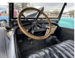
The throttle and timing adjust are on the steering wheel
