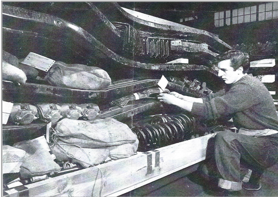
As much space as possible is being used here by packing between frames. Items, such as, springs, tubing, hubs and drums with bags of components.
